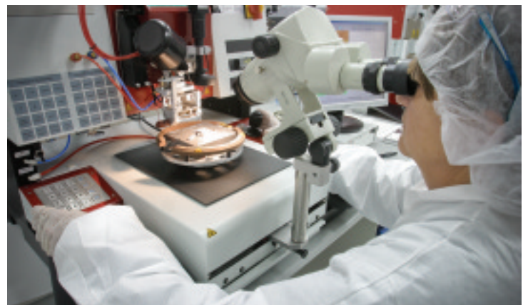
MARY ANN JOHNSON, AN ENGINEER IN RESEARCH OF SOLID-STATE LIGHTING AT OSRAM SYLVANIA IN BEVERLY, DOES WIRE BONDING OF LIGHT-EMITTING DIODES.
